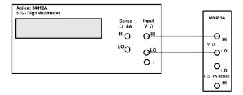
4 Program each output voltage on the M9182A/83A DMM in the order shown below. Measure this voltage with the external DMM. Compare these measurement results to the appropriate test limits shown in the table. Be certain to allow for appropriate source settling.
