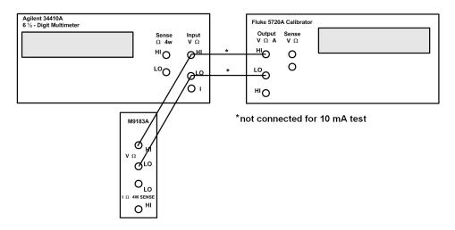
4 For the remaining output levels, connect the 34410A to the input terminals on the M9182A/83A DMM. Connect the calibrator to the input terminals of the 34410A and set the calibrator to 2-wire  $\Omega$ . Program the resistance level for each output level to generate 1 V across the 34410A input leads.
