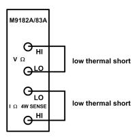
2 Now Perform the calibration process (see "Calibration Process" on page 25). Enter the calibration value of 0.00 for the calibration value (because the source is 0 V).
