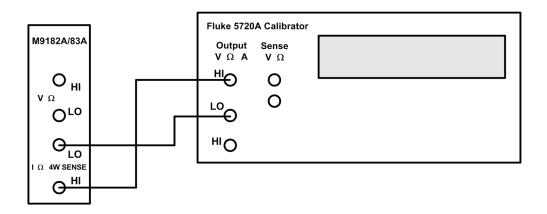
4 On the M9182A/83A DMM, select each function and range in the order shown below. Using the calibrator, provide the input shown in the table below.
