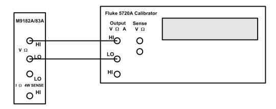
4 Select each range in the order shown below. Using the calibrator, provide the input voltage and frequency indicated. Compare the frequency measurement results from the M9182A/83A DMM to the appropriate test limits shown in the table. Be certain to allow for appropriate source settling.
