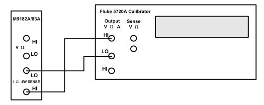
2 Apply the input signal shown in the "Input" column of the table. Enter the actual applied rms input voltage (see "Adjustments" on page 27).
